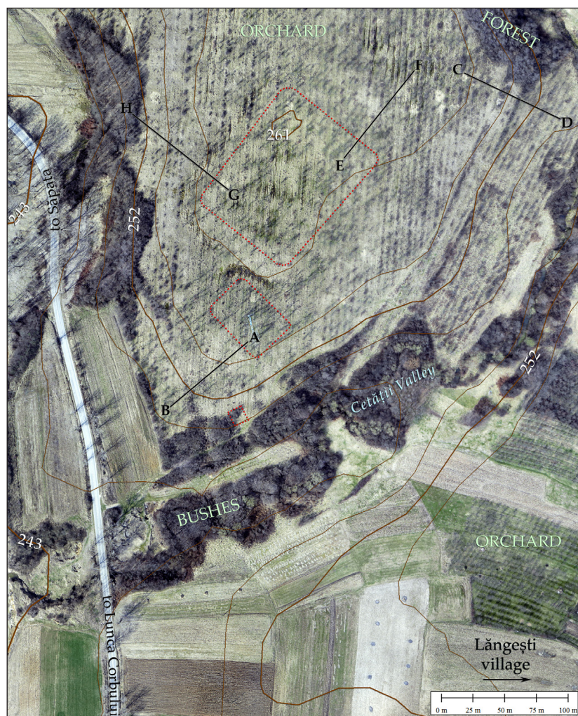
Fig. 17. Orthophoto made via UAV (res. 0.1 m), contours as in the Figure 1, and topographical sections on high resolution DEM (0.2 m), depicted at the Figure 18.
