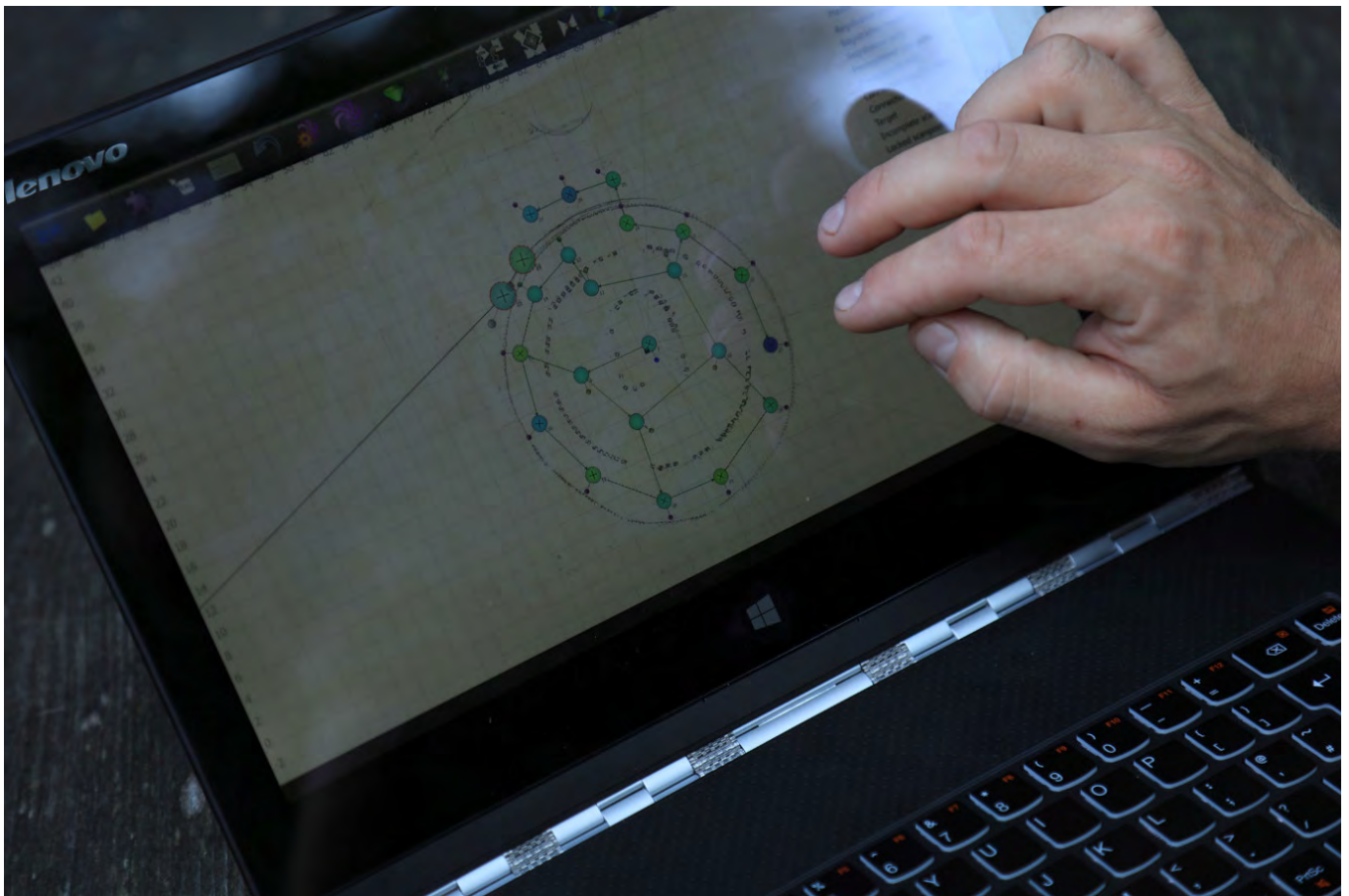
Fig. 6. Aligning point clouds using Z+F laser control software.
