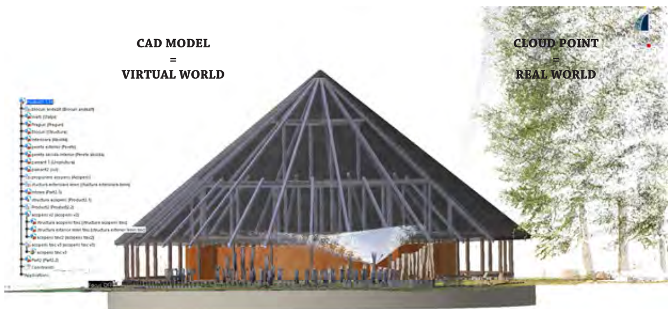
Fig. 8. The intermediary 3D model of the reconstruction proposal and the superimposed 3D scan.
