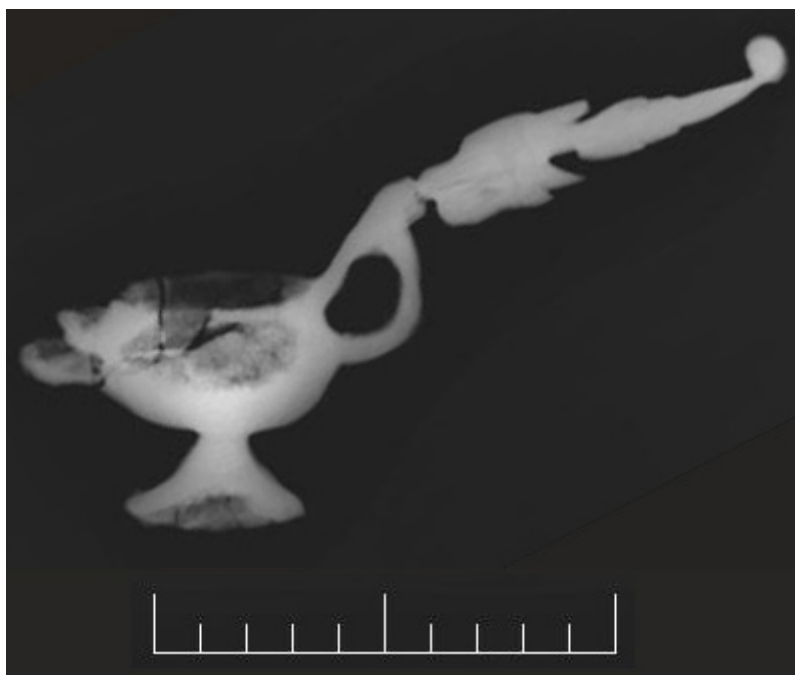
Fig. 2. Lateral X-ray image of the restored bronze lamp (courtesy of dr. Călin Marius radiologist MD).
