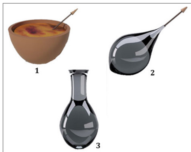
Fig. 1. Free Blowing Technique (designed by Kasım Eker in accordance with the definition of the technique).
