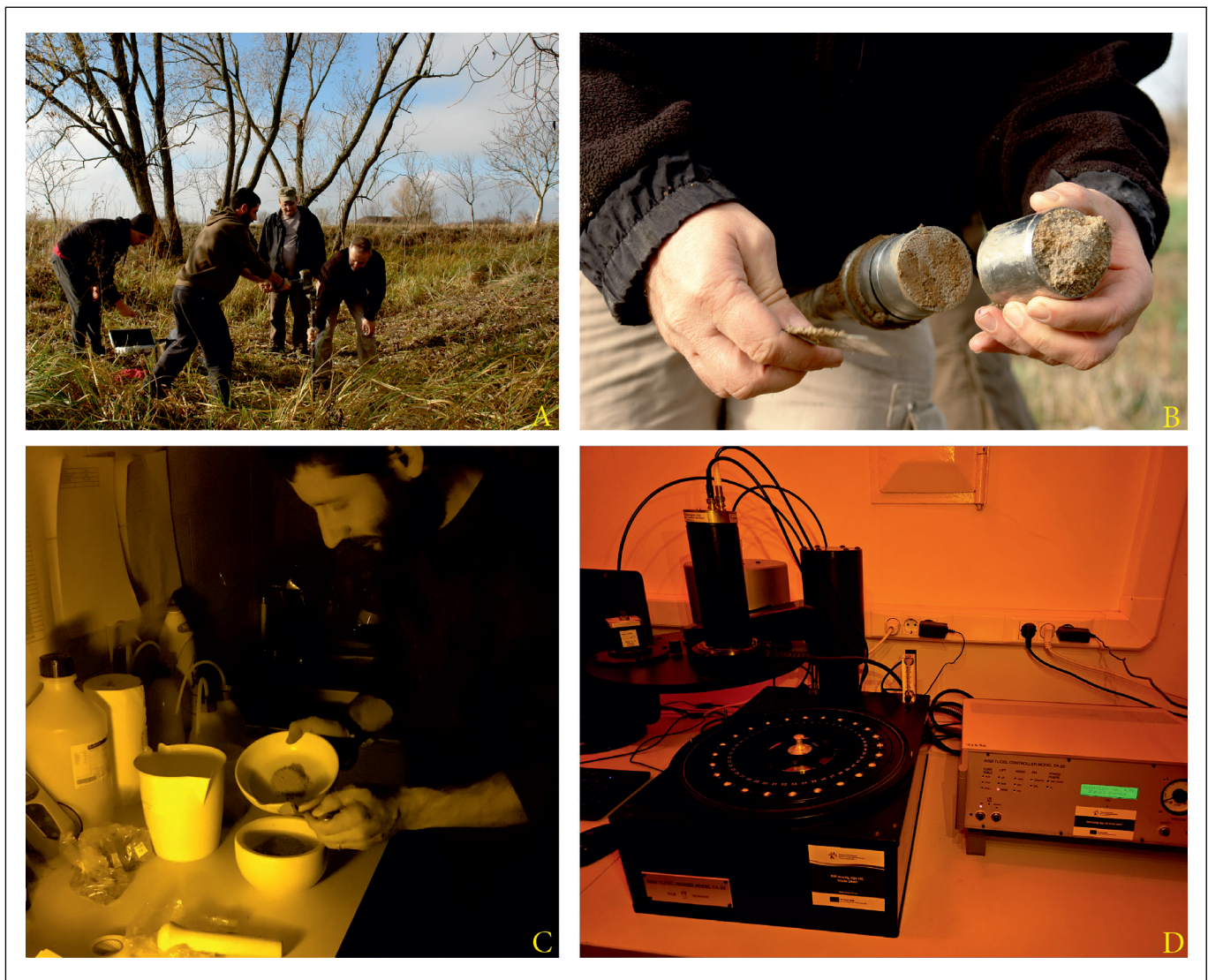
Fig. 4. OSL working flow. A: Sampling on the Pogăniș II generation, penetration of the first layers by coring; B: sample retrieval using a detachable head; C: The physical processing of the sample for separating the elements in the dark room; D: RISO TL/OSL DA-20 type luminescence reader with sample discs.
